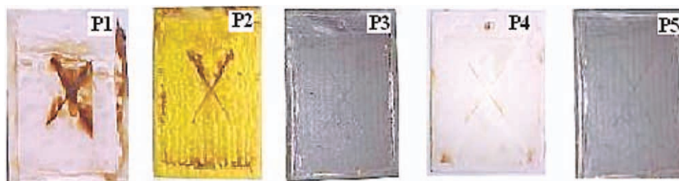
Figure 2 Photos of coated steel panels after 28 days immersion in artificial sea water. [Color figure can be viewed in the online issue, which is available at wileyonlinelibrary.com .]
